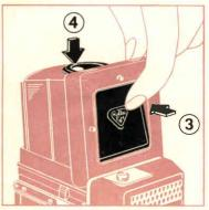
The magnifier makes accurate focusing easier. To swing it out grip the top edge of the hood with two fingers and slightly press the flap 3 inwards. Push down the magnifier 4 before closing the hood.
